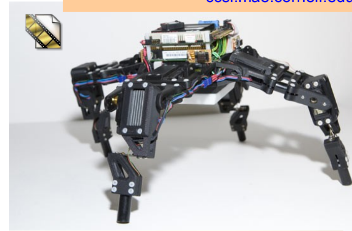
Resilient walker Gait self-teaching Functional damage compensation ccsl.mae.cornell.edu
