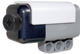
Angle incremental coder (1°) www.hitechnic.com
