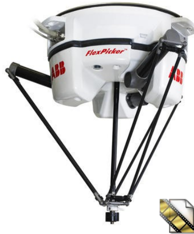
ABB IRB360 Delta 3 DOF (L3kg / R0.4m / r0.1mm) www.abb.com
