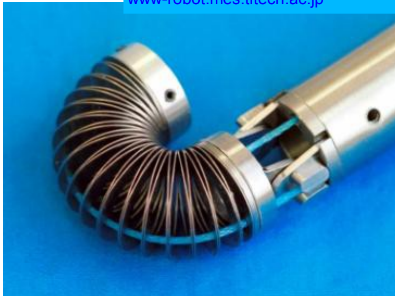
Trump orientating manipulator for laparoscopy www-robot.mes.titech.ac.jp
