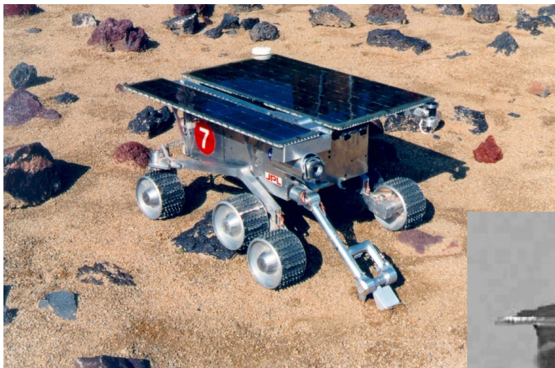
Rocky 7 Adaptative rocker-bogie structure www-robotics.jpl.nasa.gov
