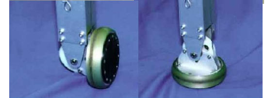
Roller-Walker (24kg, 0.5m long) Convertible wheels Dual locomotion mode: walking / roller-skating www-robot.mes.titech.ac.jp
