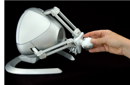
Falcon joystick 3 leg parallel mechanism www.novint.com
