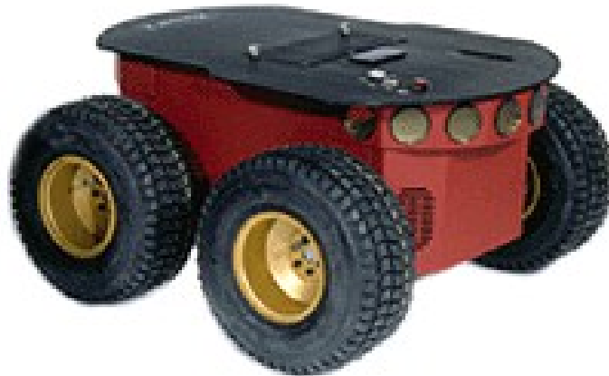
Pioneer P3-AT Skid steering simple robot www.mobilerobots.com
