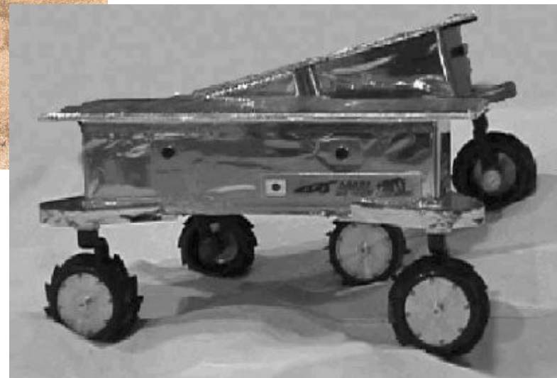
Micro5 Climbing abilities via 5 wheels www.mit.edu/~ykuroda
