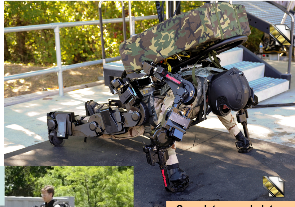
Complete exo-skeleton XOS2 Lower and upper limbs www.raytheon.com
