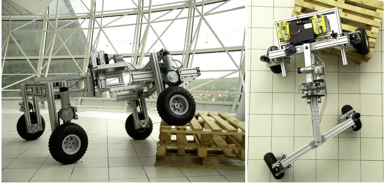
Figure 15: Full-scale OpenWHEEL i3R V3 crossing an obstacle in lateral (a) and top view (b).
