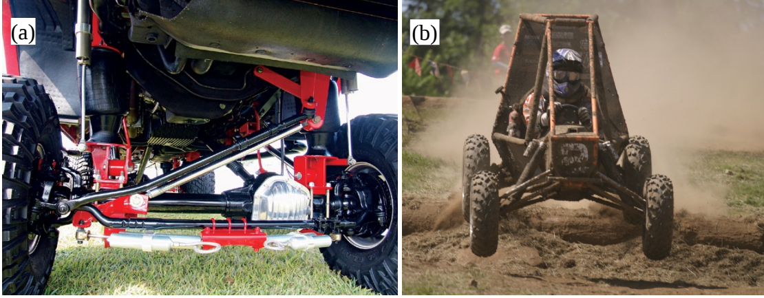
Figure 29: Examples of existing all-terrain suspensions. (a) Ford F350 4x4 rigid axle suspension. (b) Mini-Baja vehicle at Oregon State University with double wishbone suspension.
