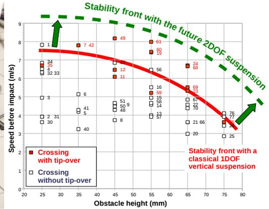
Fig.2. (a) Experimental obstacle-crossing with 1 DOF suspension. (b) Stability front of classical vehicles with dual 1DOF Z suspensions: impact speed vs. obstacle height. 2DOF XZ suspensions should extend the stability limit [2].
