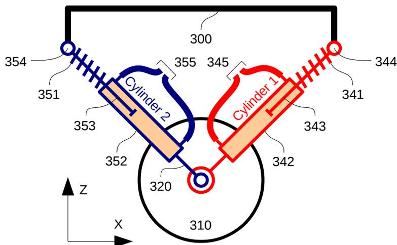
Fig.7. V3: 2D coupled 2(RPR) parallel mechanism.
