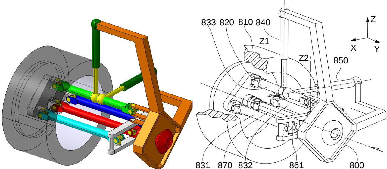
Fig.10. V8: Steering becomes decoupled from horizontal damping motion thanks to a change in the attachment point of 850 to the top bar 833.
