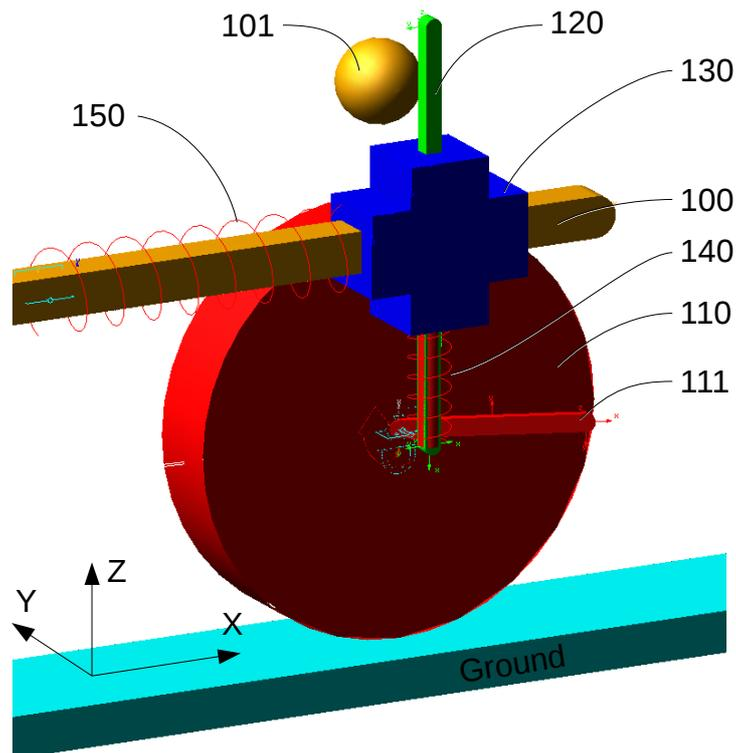
Fig.5. Version V1 of a 2DOF XZ suspension mechanism: 2D serial linkage [1].
