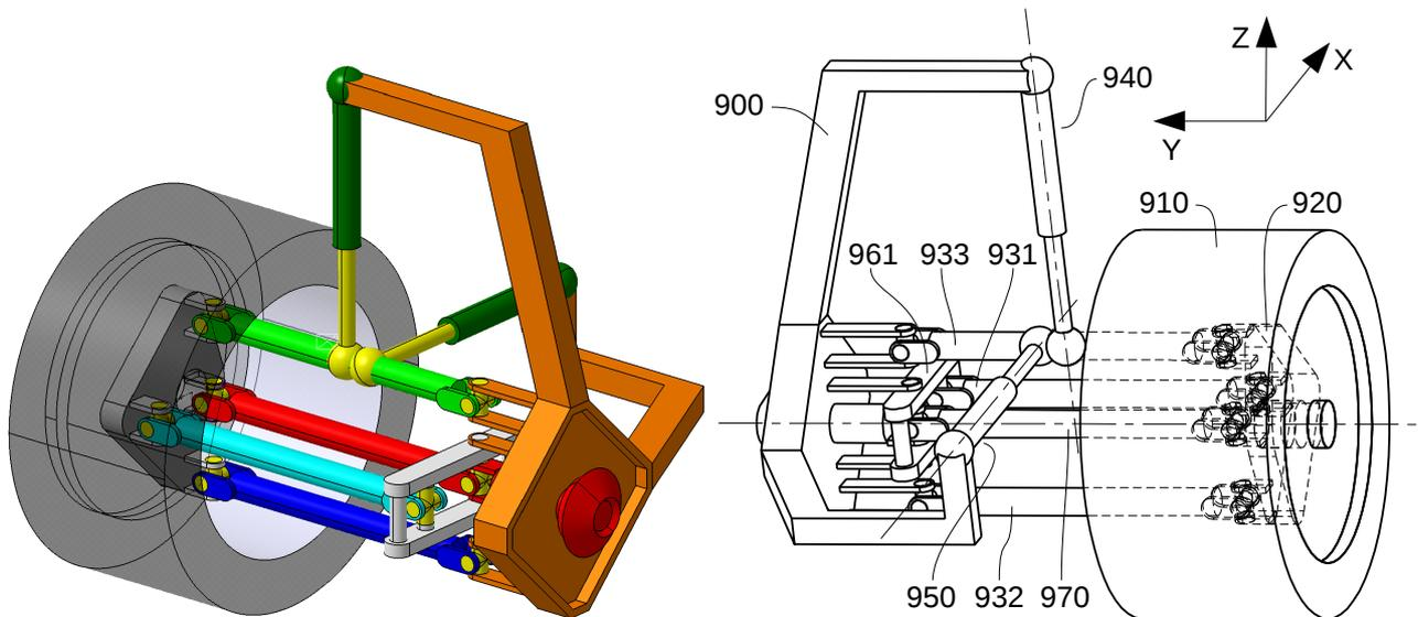
*Fig.11. V9: Variation on V8. Steering is actuated by a single arm and two bars are directly connected to the frame. This structure is very close the double triangle architecture.*
