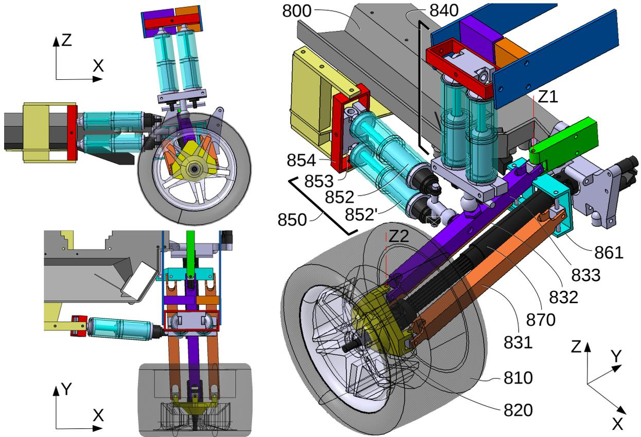
Fig.12. CAD model of V8 integrating real parts and double-damper sub-assemblies [11,12].
