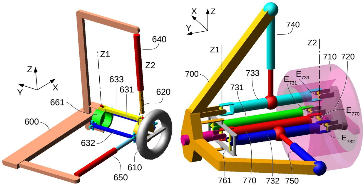
Fig.9. (a) V6: Parallel mechanism with 3DOF integrating the steering. (b) V7: the attachment points of the vertical and horizontal linkages 740 and 750 avoid any collision.
