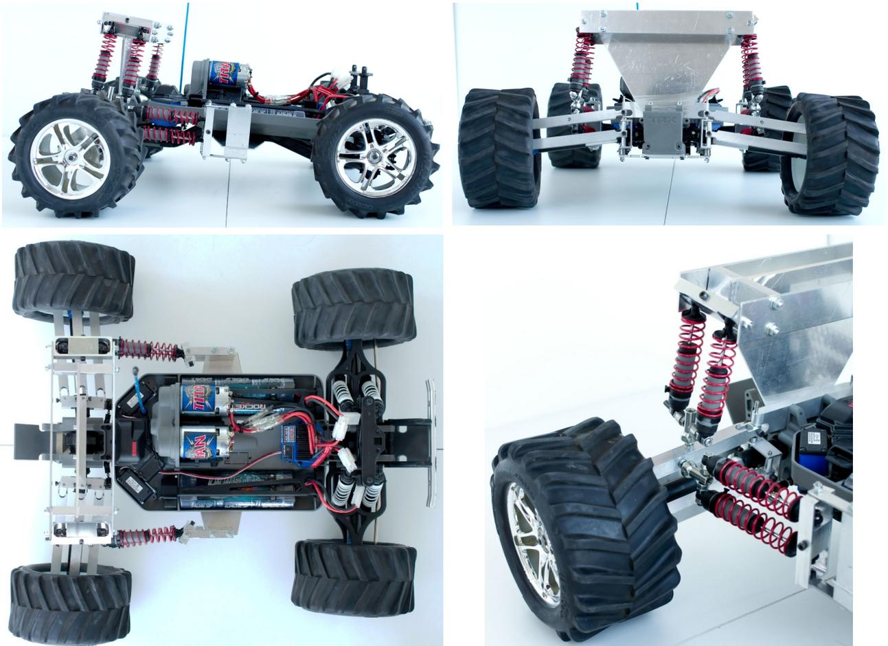
Fig.13. Mechanical implementation [11,12] of suspension V8 as the front suspension of a Traxxas E-Maxx 1:8 scale model.
