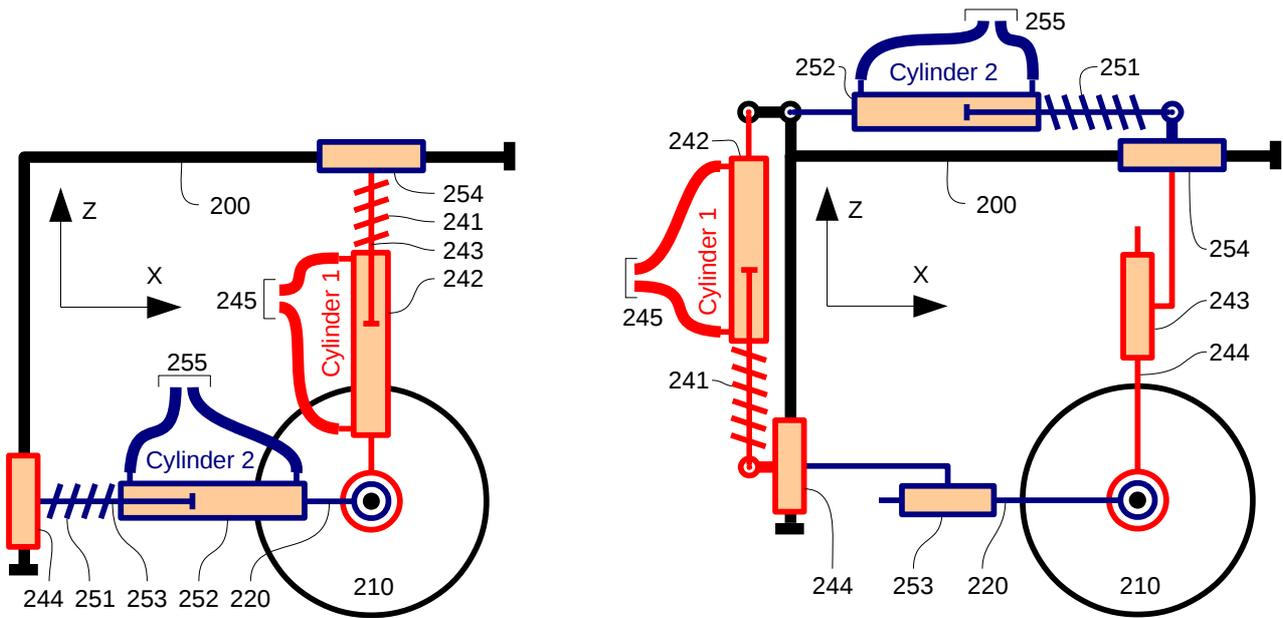
Fig.6. V2: (a) 2D parallel linkage; (b) Variant of V2 with cylinders attached to the frame.
