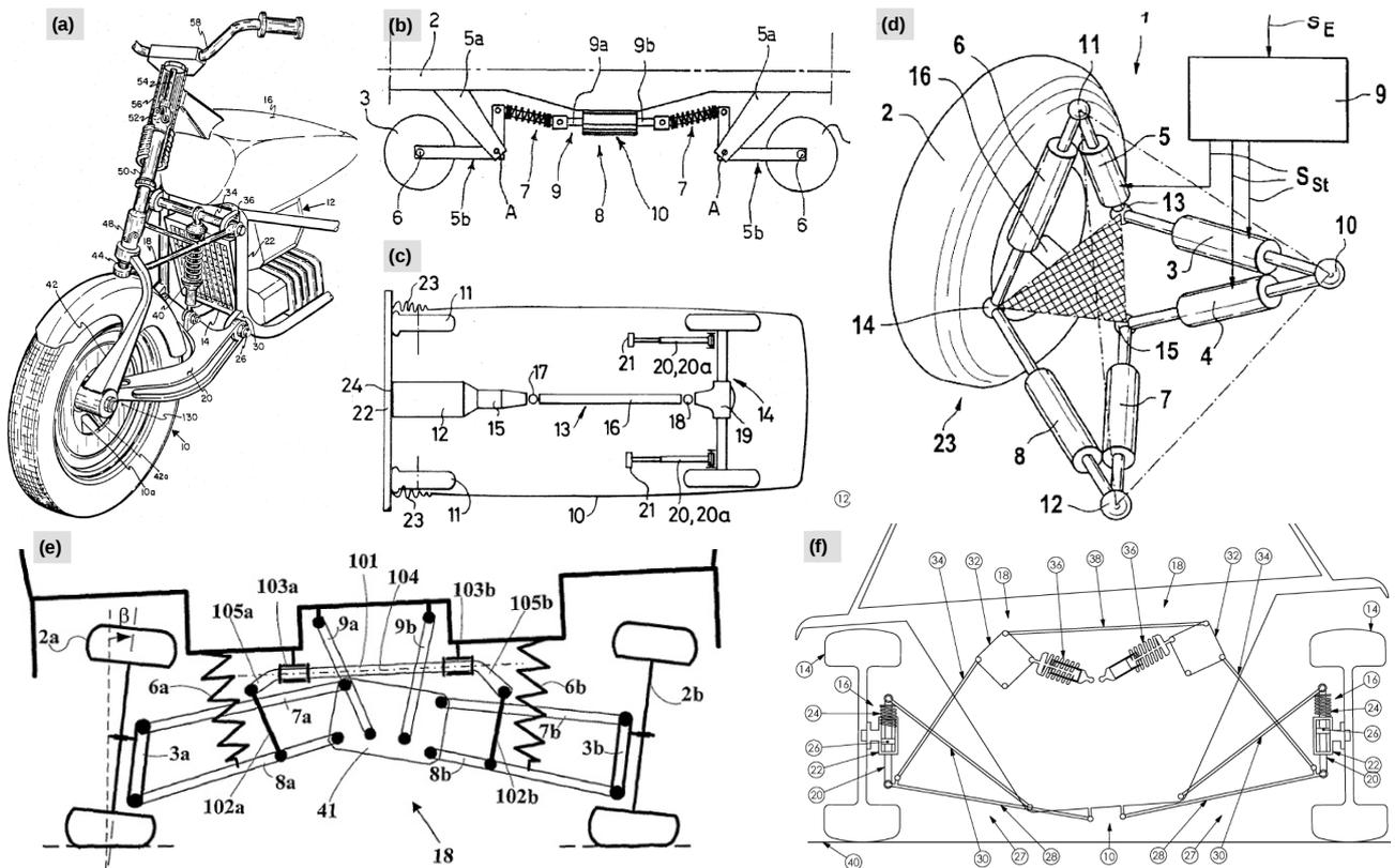
Fig.4. Selection of patents for suspension mechanisms.
