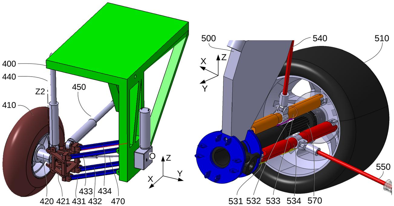
Fig.8. (a) V4: Spatial hybrid implementation [10] with four U-U parallel limbs for spherical translational suspension motions, locally uncoupled behaviour and steering capacity.
