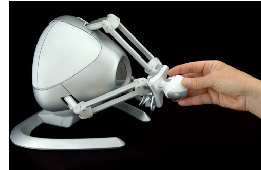
Falcon joystick 3 leg parallel mechanism www.novint.com
