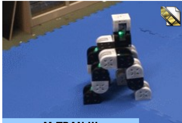
M-TRAN III Self reconfigurable robot Locomotion and Adaptation unit.aist.go.jp/is
