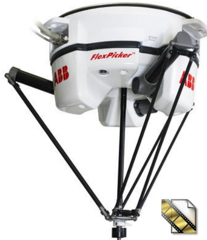
ABB IRB360 Delta 3 DOF (L3kg / R0.4m / r0.1mm) www.abb.com
