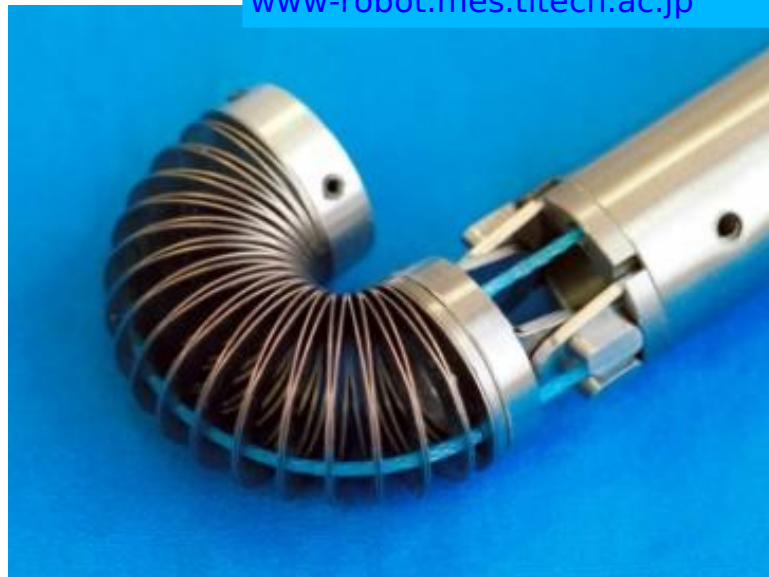
Trump orientating manipulator for laparoscopy www-robot.mes.titech.ac.jp
