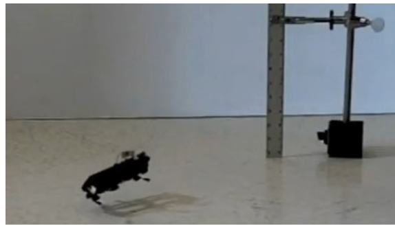
Fig. 1b) The DASH roach-like hexapedal robot bouncing after having survived a fall from a large height (Birkmeyer et al. 2009)
