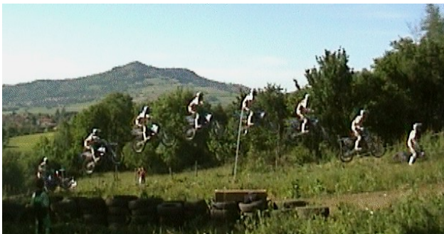
Fig. 1a) Cross-country motorcyclist performing pitch attitude correction by throttling or braking the wheels (Pouzols et al. 2006)
