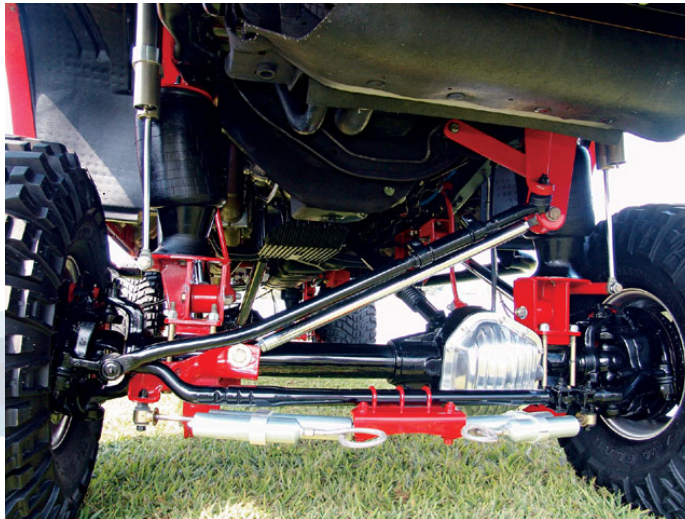
Ford F350 4x4 rigid axle suspension
