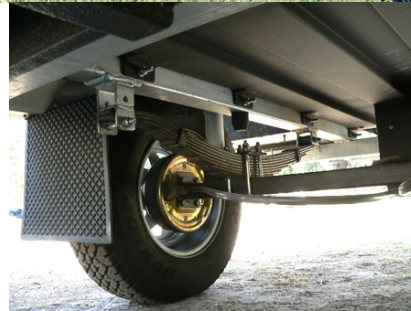
Rigid axle with leaf springs on a trailer
