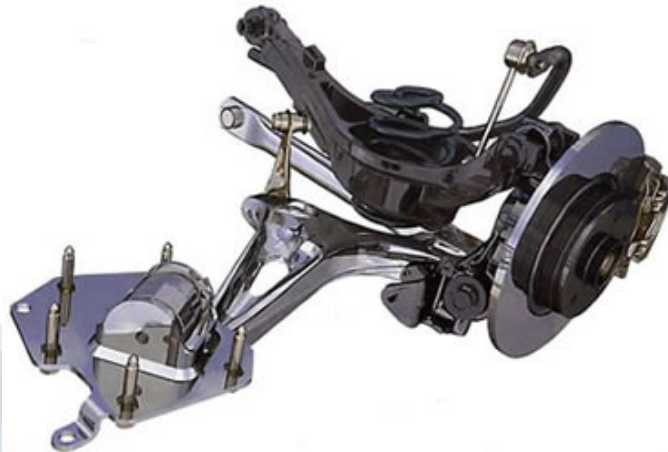
Multi-link suspension with a massive trailing-arm bushing
