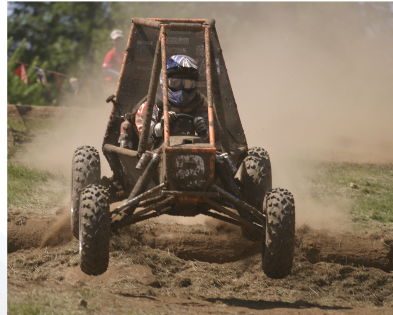
Mini-Baja vehicle at Oregon State University with double wishbone suspension
