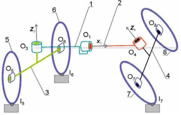
Figure 3: Kinematic diagram of OpenWHEEL i3R
