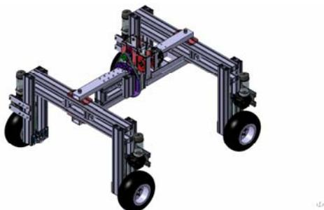
**Figure 1:** CAD model of OpenWHEEL i3R
