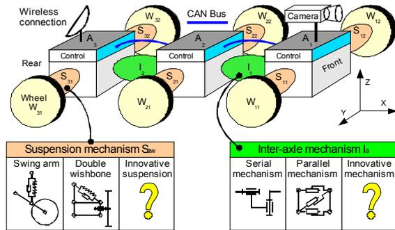
Figure 2: OpenWHEEL architecture
