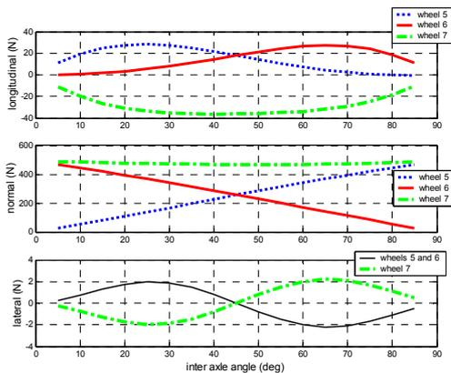
Figure 5: wheel – ground contact forces
