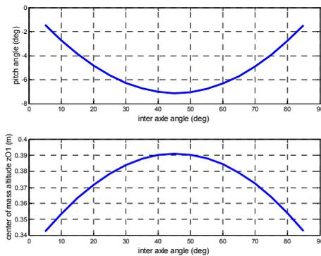
**Figure 4:** centre of mass altitude  $z_{O1}$  and pitch angle  $\theta$  as functions of inter axle angle  $\theta_{12}$
