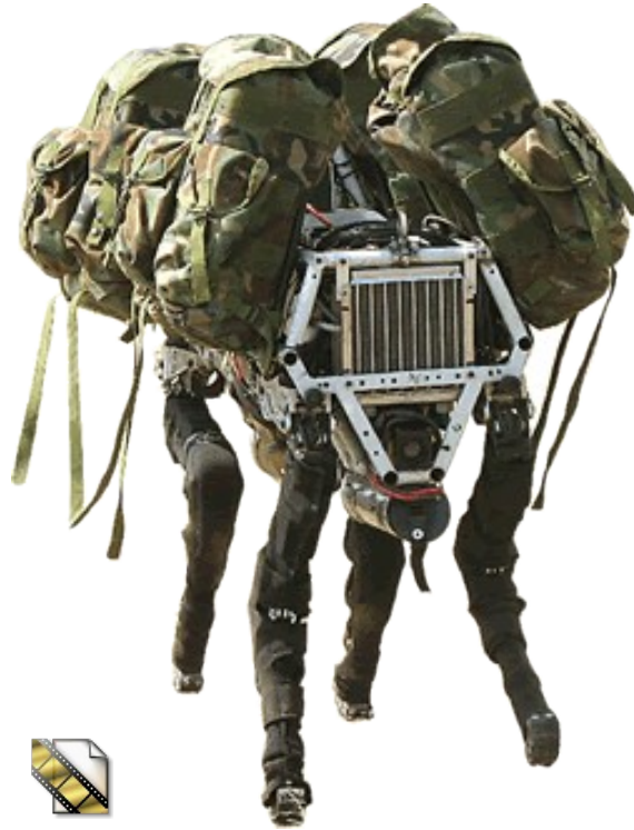
Big Dog (75kg, 1m long, 6km/h, 35° slopes, 150kg payload) www.bostondynamics.com
