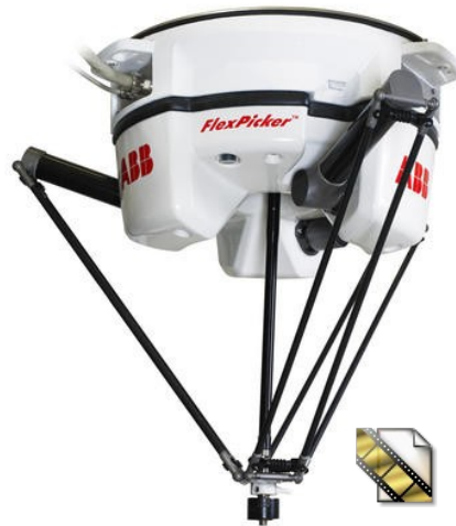
ABB IRB360 Delta 3 DOF (L3kg / R0.4m / r0.1mm) www.abb.com
