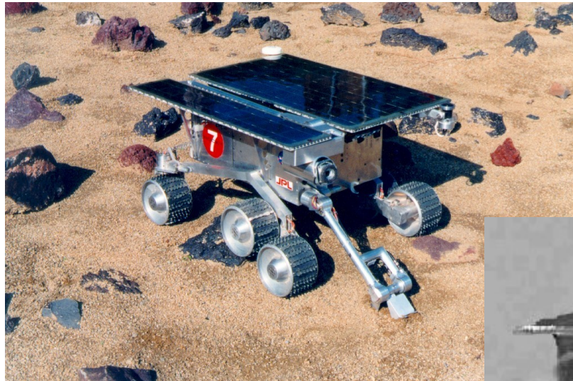
Rocky 7 Adaptative rocker-bogie structure www-robotics.jpl.nasa.gov
