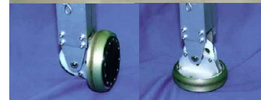
Roller-Walker (24kg, 0.5m long) Convertible wheels Dual locomotion mode: walking / roller-skating www-robot.mes.titech.ac.jp
