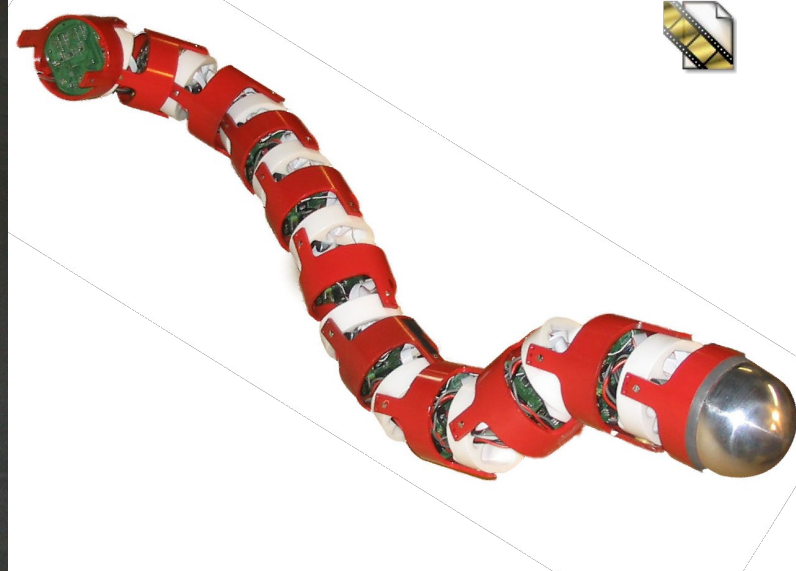
Aiko 7kg, 1.5m long, 20 DOF, 2.5 Nm Obstacle-aided locomotion, slidewinding www.sintef.no
