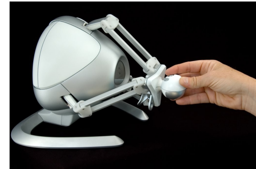
Falcon joystick 3 leg parallel mechanism www.novint.com
