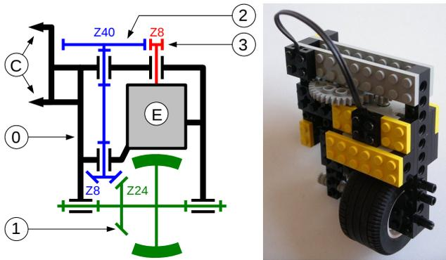
Fig. 5. A wheel sub-assembly with actuator and speed reducer.
