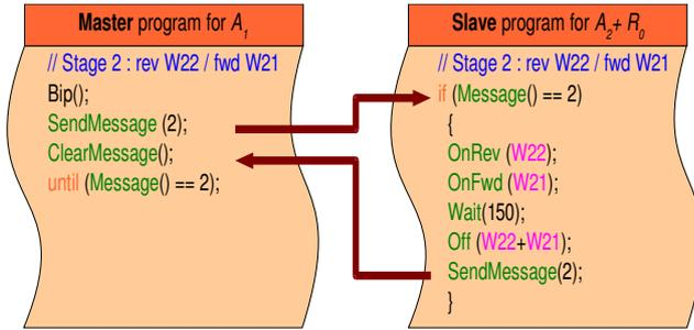
Fig. 8. A sample from the master-slave programs that control the axles.
