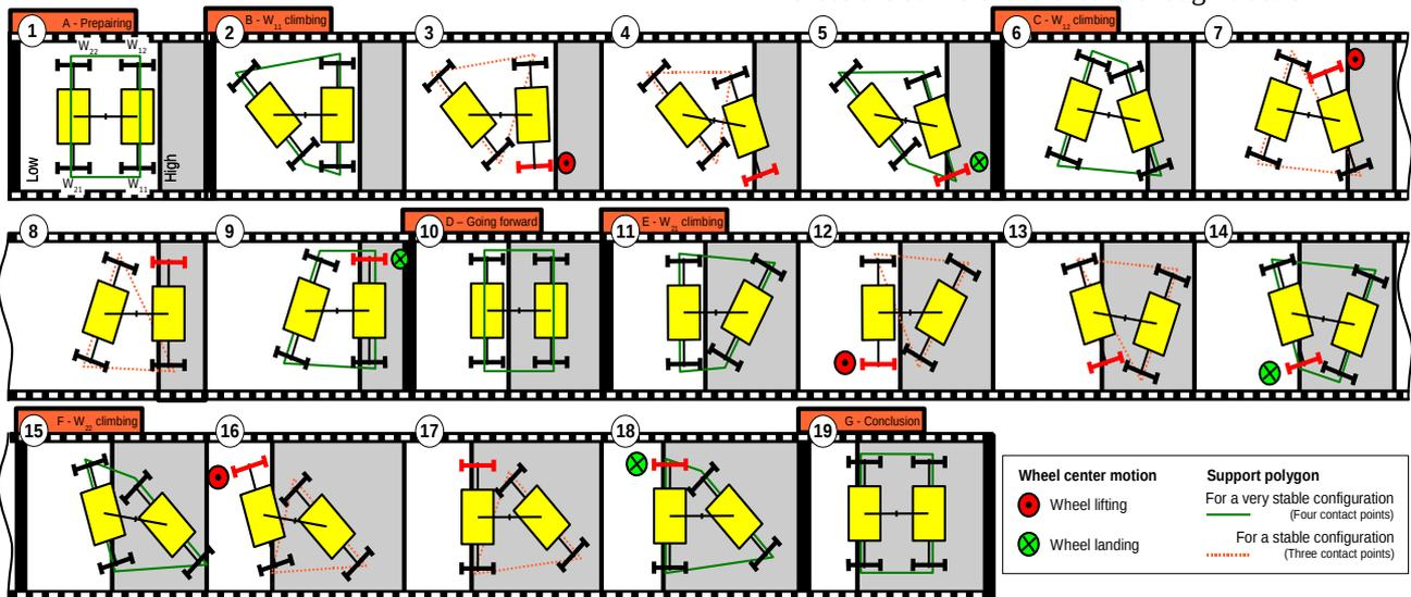
Fig. 4. 2D modeling of a climbing process in nineteen phases.
