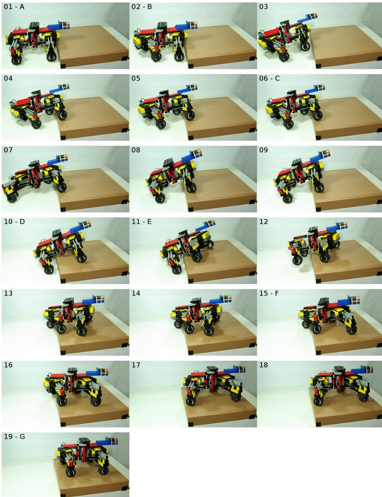
Fig. 9. Experimenting the climbing process in nineteen phases on an actuated and autonomous reduced model of the OpenWHEEL i3R.
