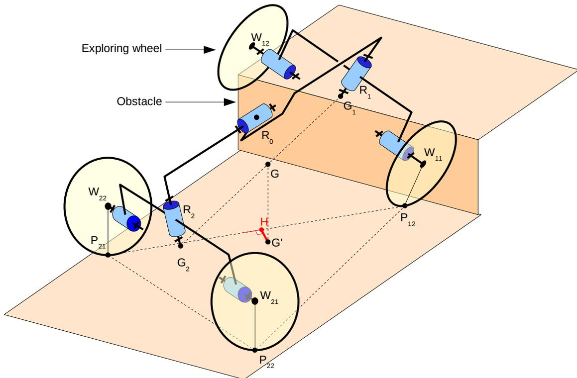
Fig. 2. The concept of exploring wheel (here  $W_{12}$ ).
