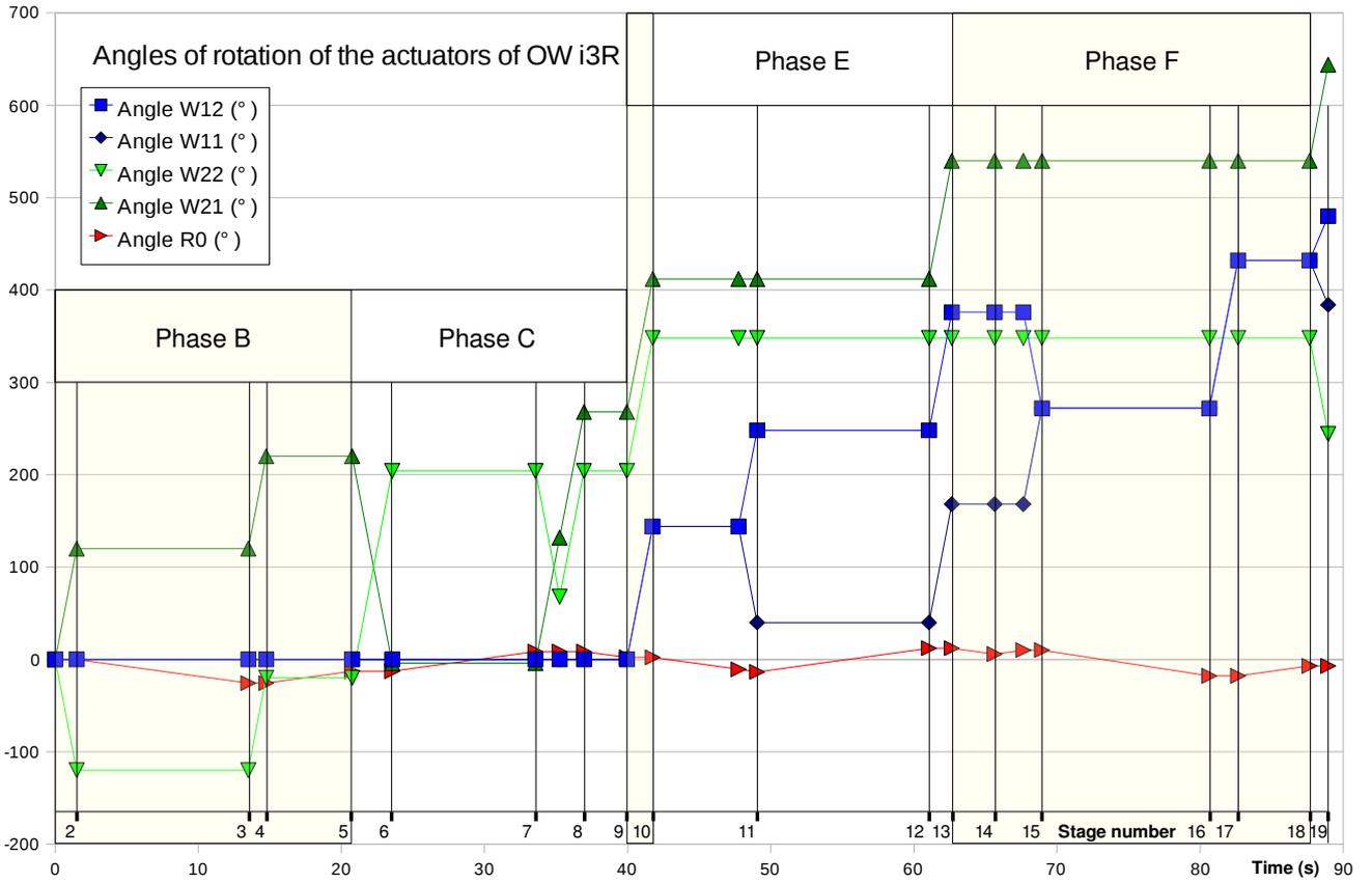
Fig. 10. Control laws of the five actuators of OpenWHEEL i3R.
