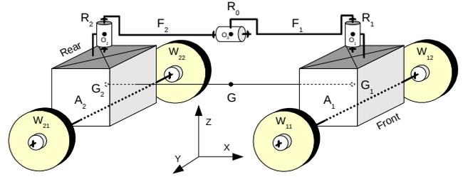
Fig. 1 OpenWHEEL i3R mobile robot structure with two axles  $A_a$ .
