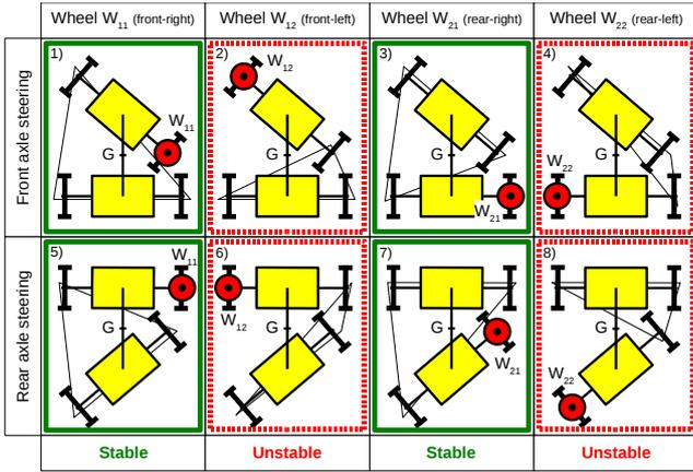
Fig. 3. Stability on 3 wheels occurs if the lifted wheel is inside the turn.
