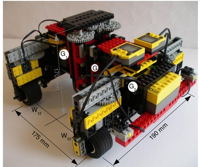
Fig. 7. The assembled reduced model with dimensions.
