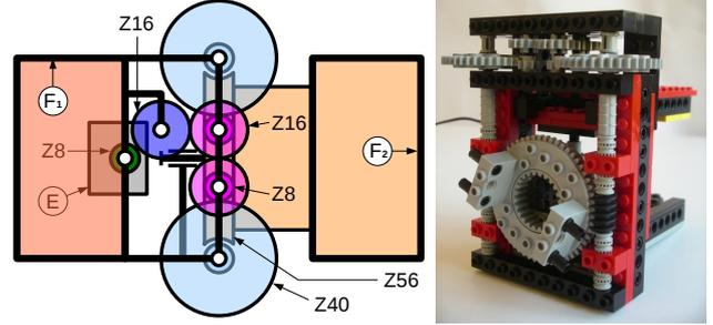
Fig. 6. Structure of the inter-axle speed reducer of joint  $R_0$ .
