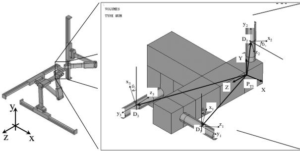
Fig.3: Moving platform of the Isoglide3-T3
