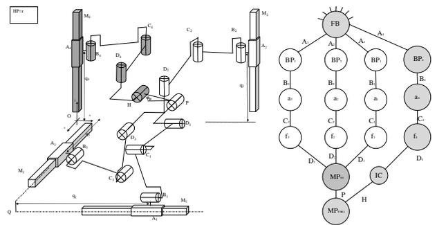
Fig.1: Kinematic scheme and graph of the Isoglide4-T3R1
