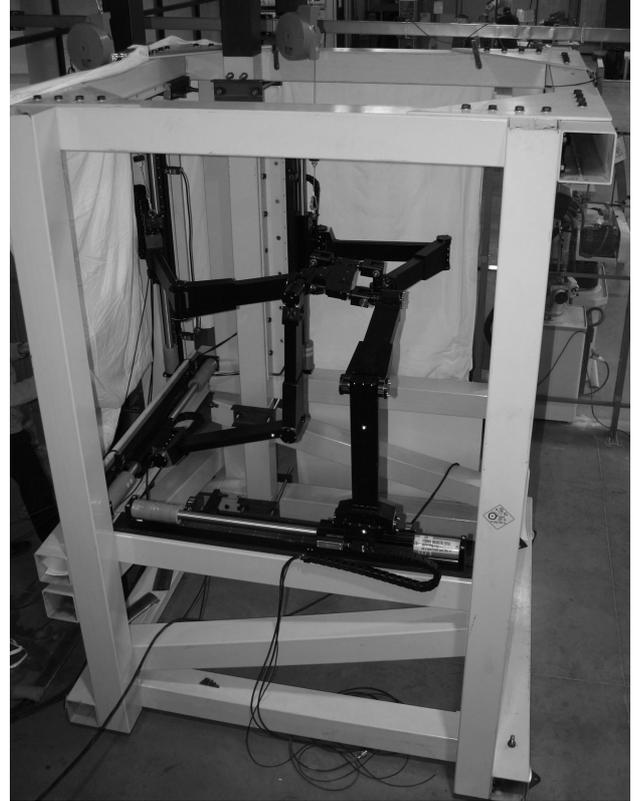
Fig.5: real prototype of the Isoglide4-T3R1
