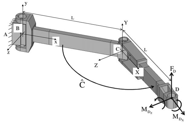
Fig.2: CAD model of an isolated leg
