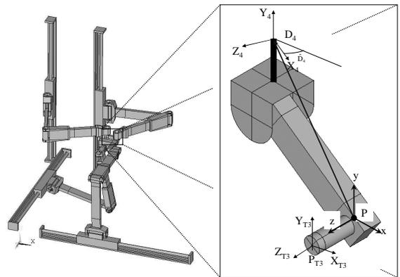
Fig.4: Moving platform of the Isoglide4-T3R1
