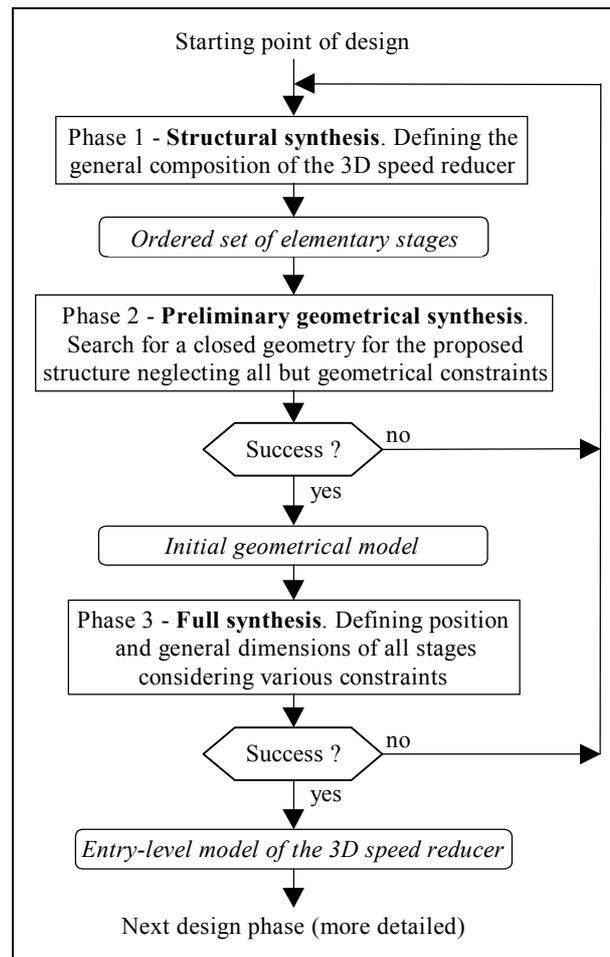
**Fig. 1.** Preliminary design process of 3D Speed Reducers
