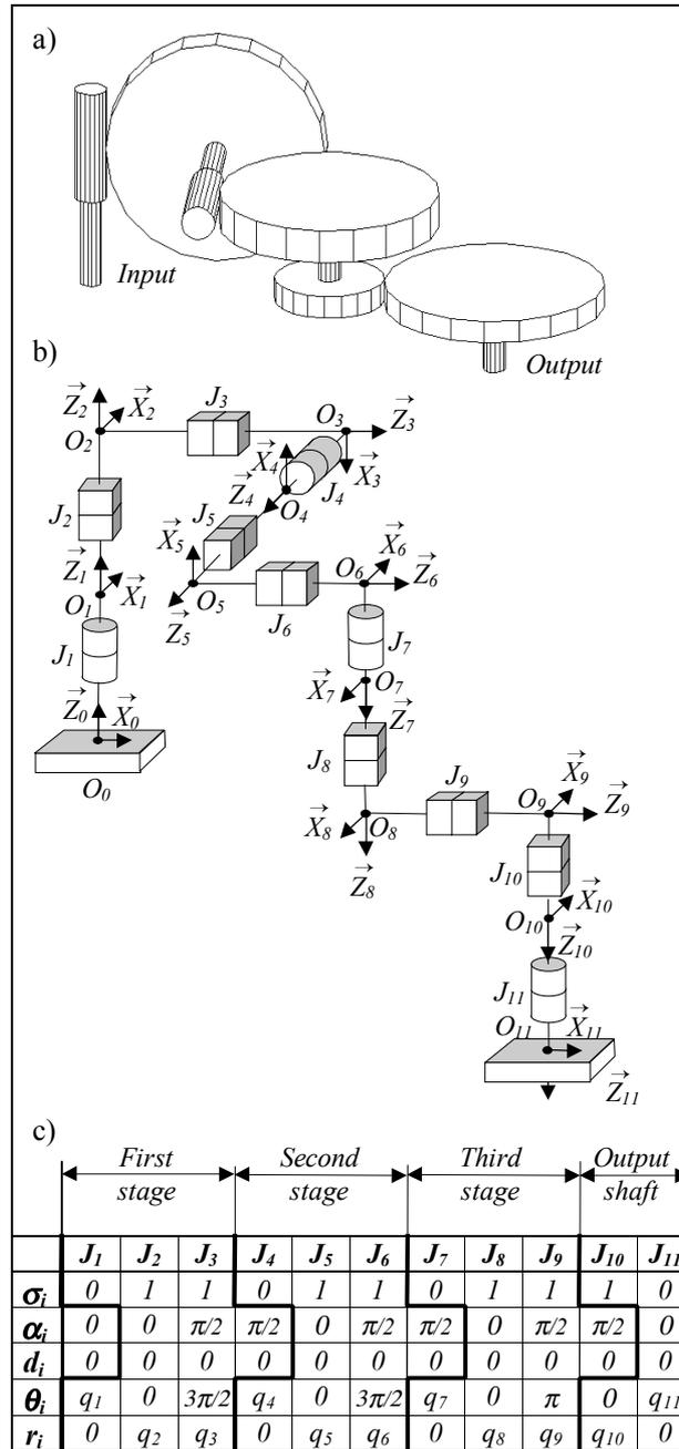
Fig. 9. 3D.S.R example and its whole geometrical model
