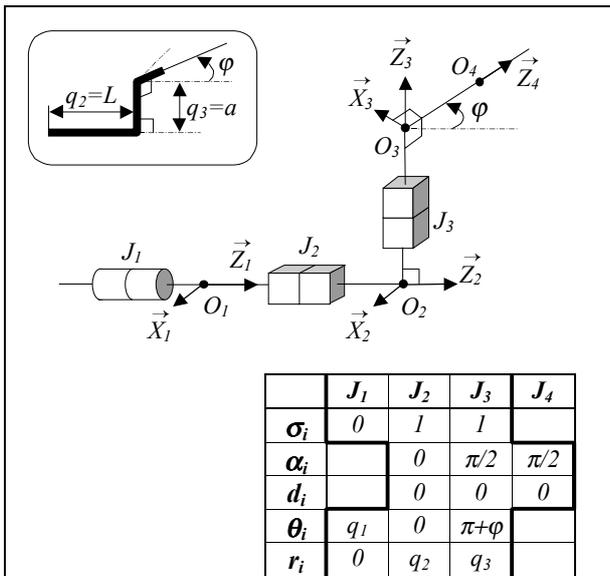
Fig. 7. Geometrical model for non concurrent shaft stages
