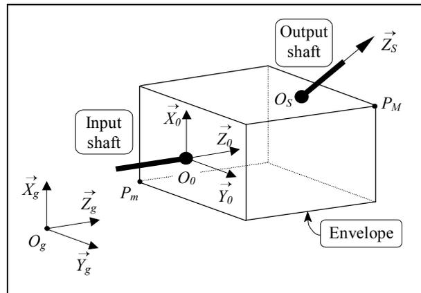
Fig. 4. Geometrical specifications
