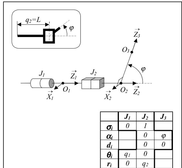
Fig. 8. Geometrical model for concurrent shaft stages
